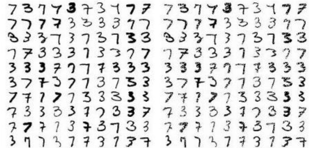
Fig. 2. Adversarial construction on MNIST dataset of 3s and 7s such that each example has a minimal number of pixels altered to mislead the discrimination between the two sets among the ten classification bins.
